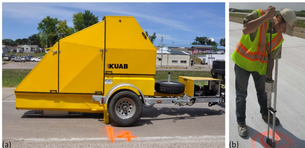
Figure 3.2. In situ testing procedures: (a) Kuab FWD setup with 300 mm diameter loading plate and (b) DCP with 2m extension rods.
